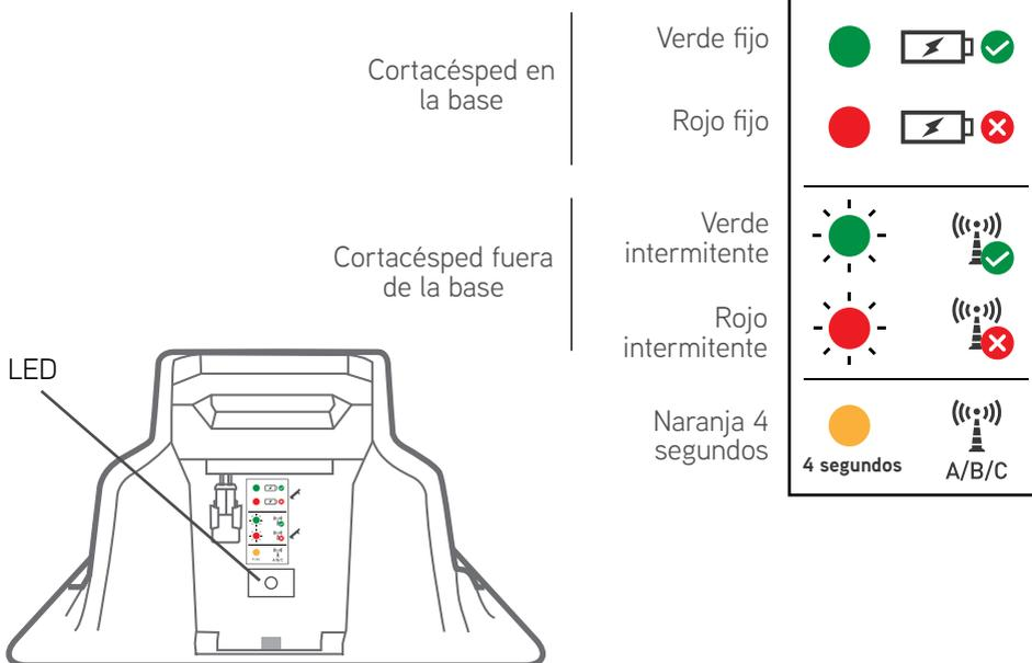
The diagram shows the back of the base station with a label 'LED' pointing to a panel of indicator lights. The legend on the right explains the following states:
