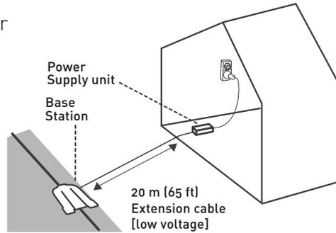
Connect the DC cable from the Power Supply unit to the 20 m (65 ft) extension cable.
