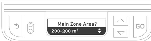
Enter the size of your Main Zone area. When you see the message “Test wire position,” it means your mower is ready to test. Press GO. It will start driving.
