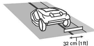
When the edge is a wall (more than 2 cm/1" above the ground level), use the longer distance of the RoboRuler.
