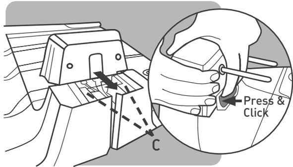
Feed the Extension Cable into the Power Supply unit.
