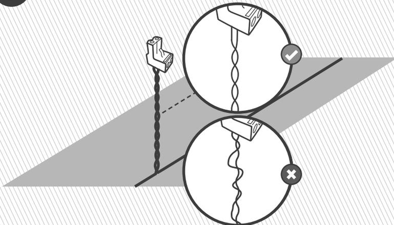
Strip back 5 mm (0.2 in) of insulation from the wire ends, insert the twisted wire into the connector and secure it using a small flat screwdriver.
