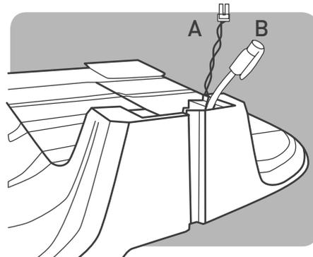
Attach the Perimeter Wire connector to point A on the Base Station's head. Attach the 20 m (65 ft) extension cable to point B on the Base Station's head.
