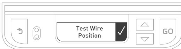
Walk alongside as the mower tours the perimeter. At the end of a successful tour the message “Wire test succeeded!” will be displayed and the mower will reenter the Base Station. Press GO.
